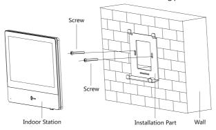
Figure 5-2 Installing the Plate
