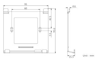
Figure 5-1 Wall Mounting Plate
