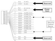
Figure 4-1 Wiring Description (Alarm Input Device)
